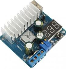
**DC-DC Boost Converter CC CV 3...35V**
