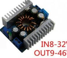
**DC-DC Boost module 8-32V step-up to 9-46V 150W**
